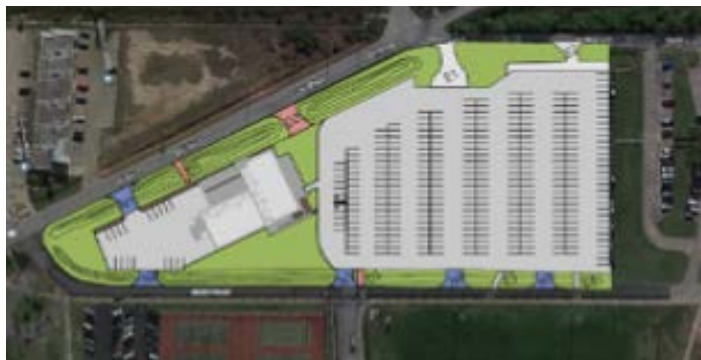
| Site plan for new supplemental utility plant
