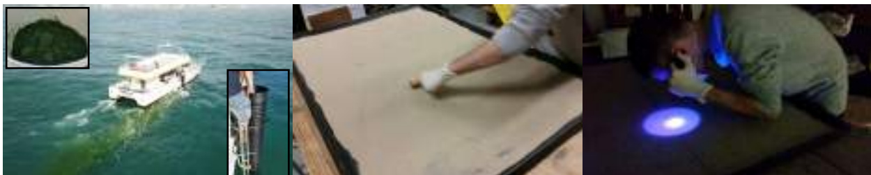
Figure 1. Images demonstrating offshore deployment (left), and preparation (middle) and quantification (right) of the sand tracer under a blue, UV torch light with bulk sediment sample collected from the SPI nearshore berm placement area. The photo of the offshore tracer deployment was taken by City of South Padre Island on August 15, 2018. The photos of a former Research Experiences for Undergraduates (REU) student (Texas A&M Ocean Engineering – Galveston) performing the sediment laboratory analysis were taken on November 12, 2018.
